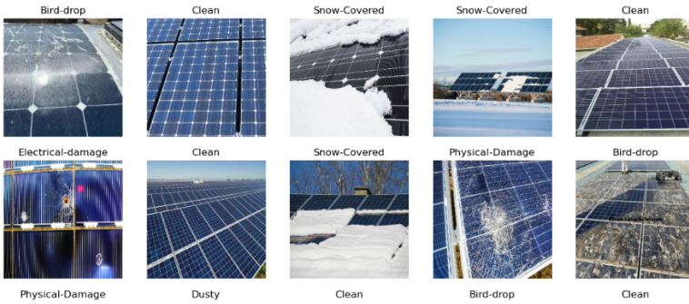
Fig 9. Failure detection of Solar panels (Kaggle, 2025)
