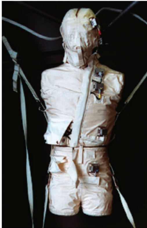
Figure 6. Radiation dosimetry model containing more than 300 radiation sensors used by NASA (Rask et al., 2010).
