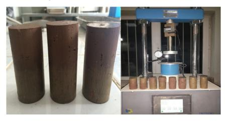
Figure 2.Specimens and unconfined compression test device
