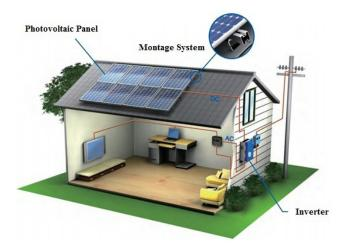
Figure 4: Example of Electricity Generation in a Residence Using a PV System.
