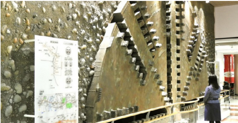
Figure 5. Tunnel Boring Machine (TBM) Head. (URL-5)
