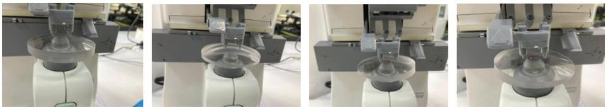
**Figure 9.** Focimeter measurement of prismatic eyeglasses.
