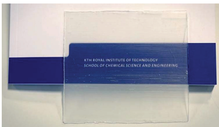
Figure 1. Transparent wood sample created at the KTH Royal Swedish Institute of Technology (Katunský et al. 2019).
