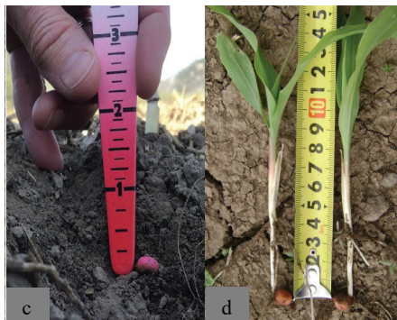
Figure 13. Calibration for planting depth in field conditions; before emergence (c), after emergence (d)
