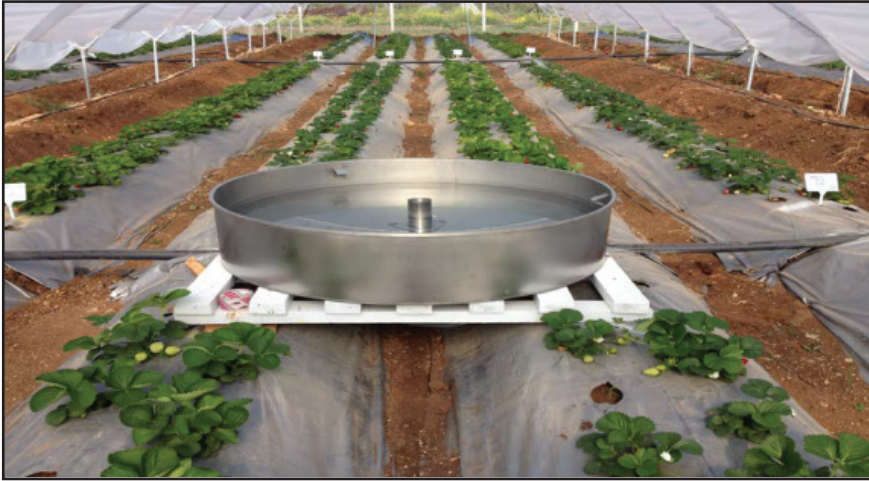
Photograph 3. Class A evaporation pan
