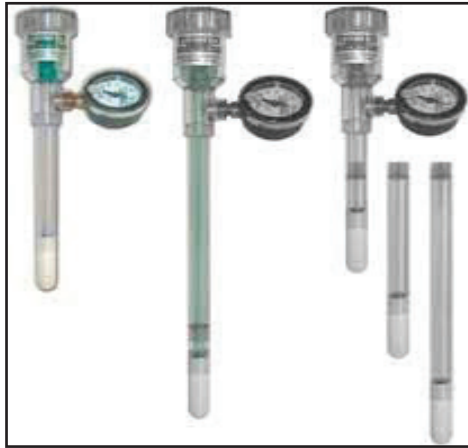
Photograph 2. Tensiometers that indirectly determine the soil water content
