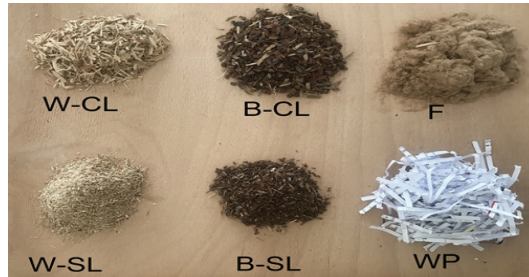
Figure 1. W-CL : Wood core layer, B-CL : Bark core layer, F : Fiber, W-SL : Wood surface layer, B-SL : Bark surface layer, WP : Waste paper.
