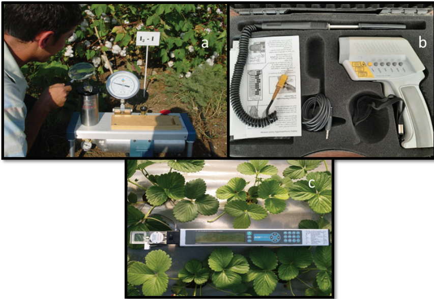
Photograph 3. Equipment used in determining the irrigation time; a. leaf water potential meter, b. infrared thermometer, c. stomal conductance and photosynthesis meter.
