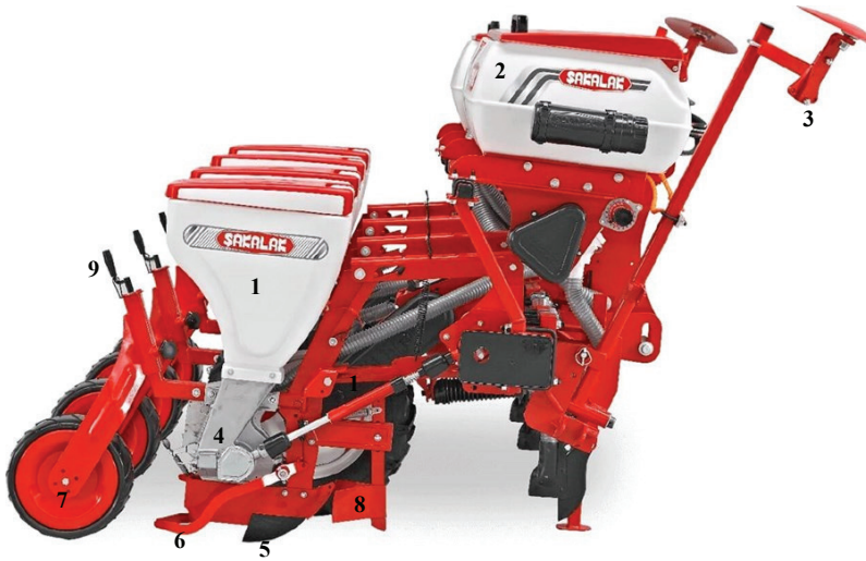
Figure 1. Vacuum precision planter; seed boxes (1), fertilizer boxes (2), marker (3), seed metering system (4), furrow opener (5), closer (6), pressure wheels (7), row cleaner (8), and depth adjustment lever (9) ( http://www.sakalak.com )
