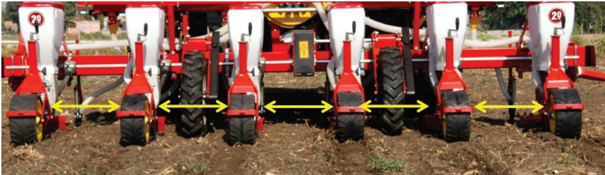
Figure 5. Inter-row spacings in vacuum precision planter
