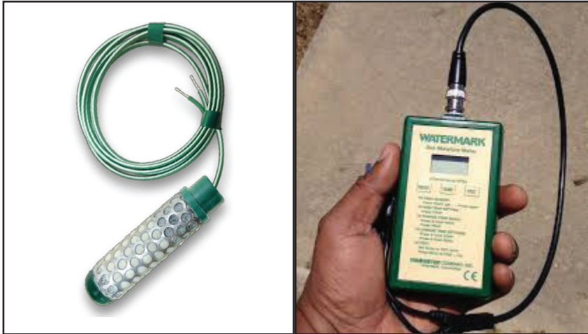
Photograph 1. Electrical resistance blocks measuring soil water content.
