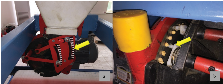
Figure 9. Seed singulation adjustment (a) and singulator (b)
