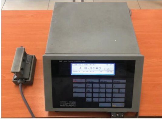
Figure 2. QTM-500 thermal conductivity measuring device (Sözen, 2019).
