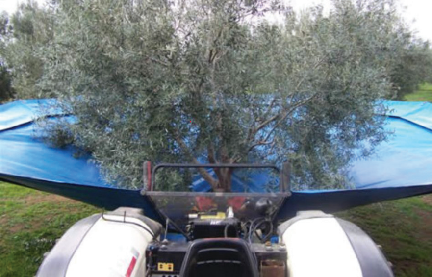
Figure 1. Umbrella-type trunk shaker (Anonymous a, 2021)
