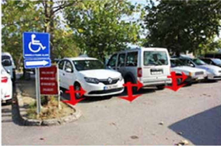
Disabled car parking in front of medical school - there is no access corridor
