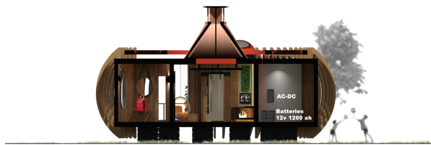
Figure 6. Section of energy generation and storage from solar panels (İmert, 2017).
