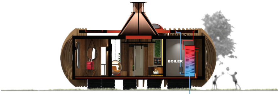
Figure 4. The section of underfloor heating with boiler (İmert, 2017).
