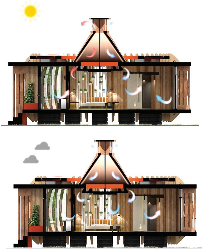
Figure 3. The working principles of wind catcher during day and night (İmert, 2017).
