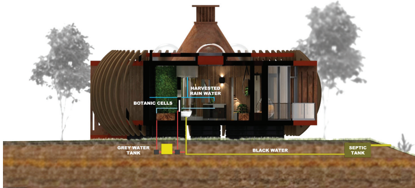
Figure 8. Section of waste water management system (İmert, 2017).
