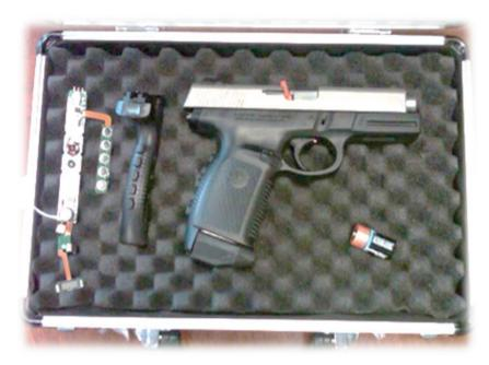
Figure 5. A biometrically controlled prototype developed by Smith & Wesson
