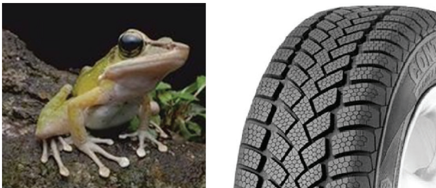
Figure 6: Biomimetic tire inspired by frogs toe pads [11,12].
