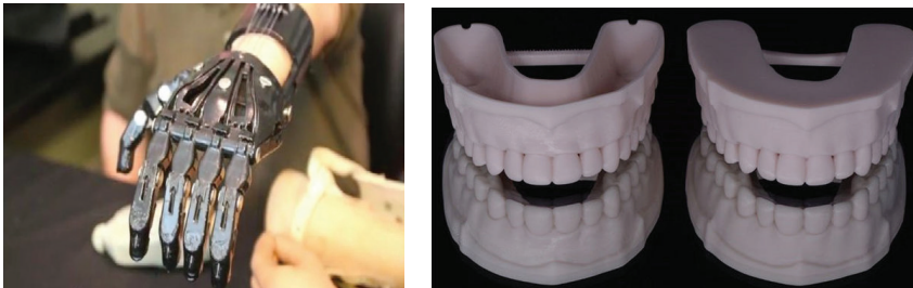
Figure 9. Prosthetic arm (Mills, 2015) and teeth (Rungrojwittayakul et al., 2020) produced with 3D printer technology
