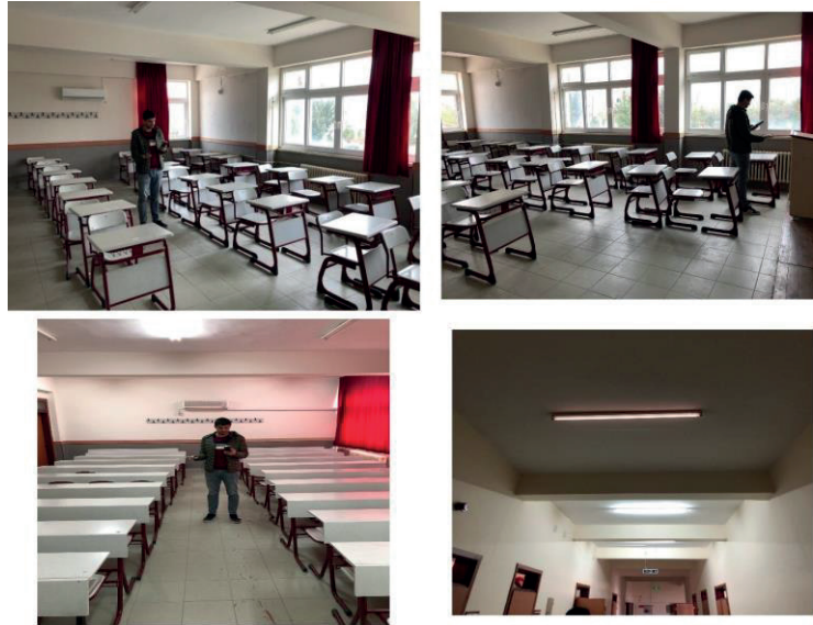
Figure 2. Images of the illuminance measurements carried out in the classrooms and corridors
