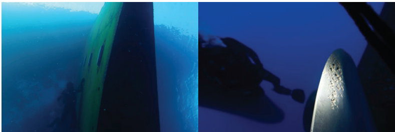
Figure 2: The hull surface is cleaned by divers.
