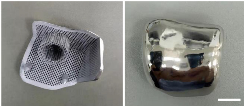
Figure 4. SLM CoCr Based Ankle Joint (Lu et al., 2023)
