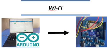
Figure 4. Over-The-Air (OTA) programming on Wemos D1 Esp8266 Wi-Fi Card
