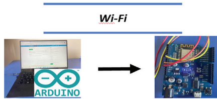
Figure 4. Over-The-Air (OTA) programming on Wemos D1 Esp8266 Wi-Fi Card
