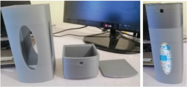
Figure 5. 3D printed polymer container parts of the automated hand sanitizer.
