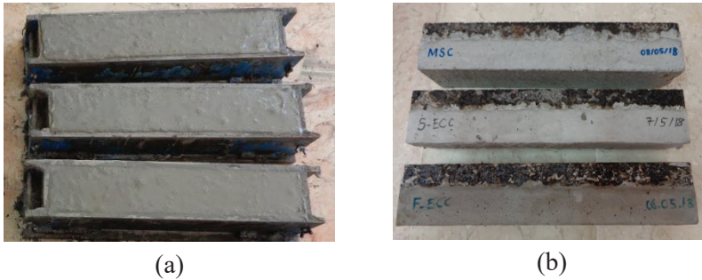
Figure 1. Production of the overlay material/asphalt concrete composite beam specimens
