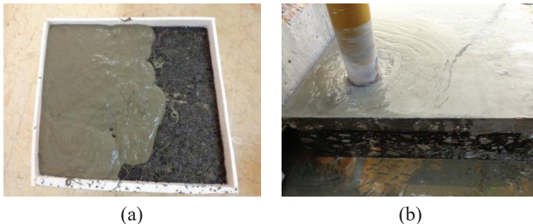
Figure 2. Production of the direct pull-off test specimens
