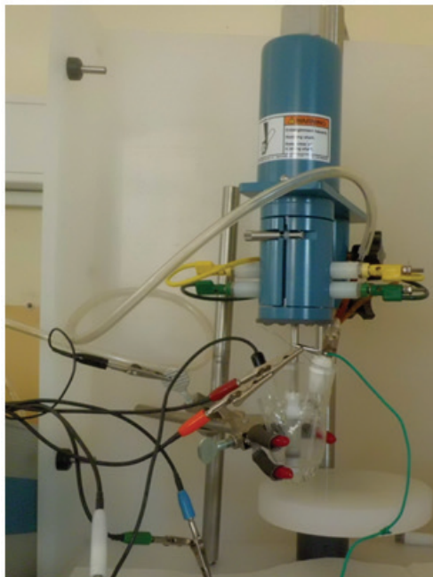
Figure 3. Three electrode cell consisting electrochemical sensor studies.
