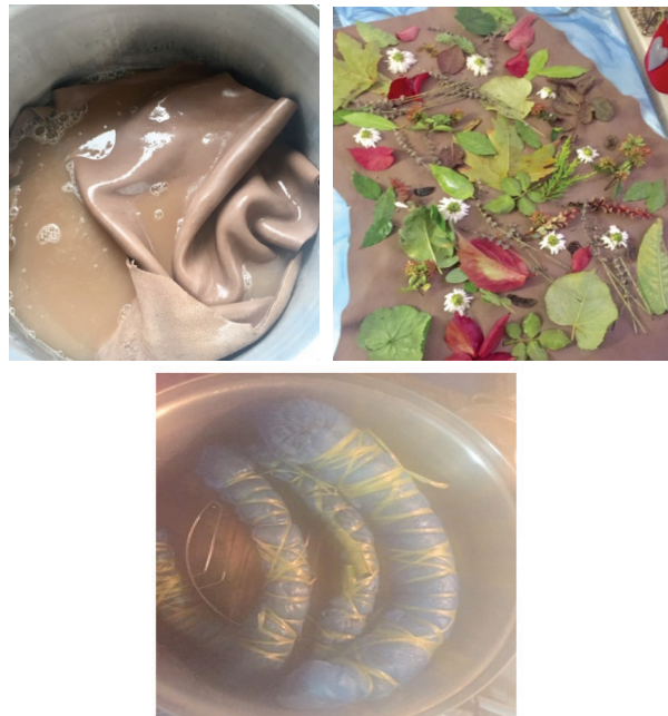
Figure 4. Vegetable tanned leather: soaking, placement of plants and hot roll process
