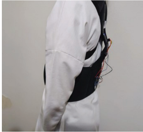
Figure 18. User is warned by vibration and sound.
