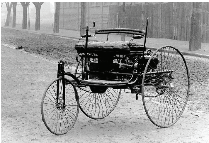
Figure 3. The first ICE car (Benz Patent-Motorwagen), designed by Carl Benz in 1885 (URL-3).
