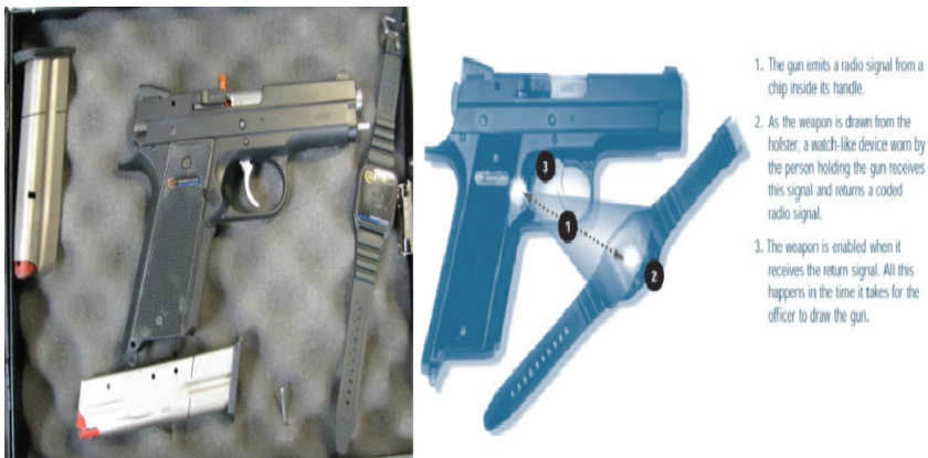
Figure 4. Prototype and Working Principle Developed by Colt's Manufacturing Company
