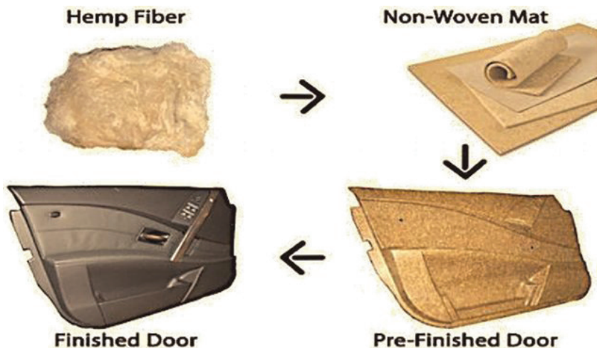
Figure 3. The use of hemp fiber in automobile door [15]
