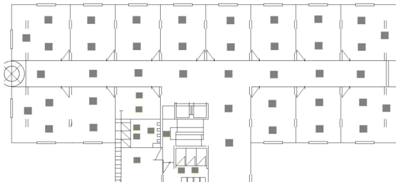
Figure 2. Office building lighting floor plan
