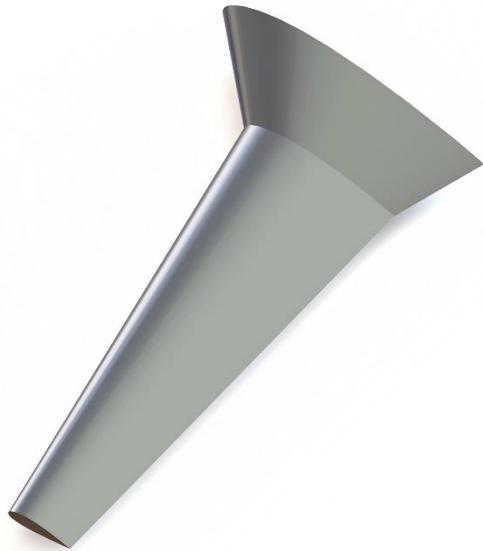
Figure 3. The solid model of the considered aircraft wing
