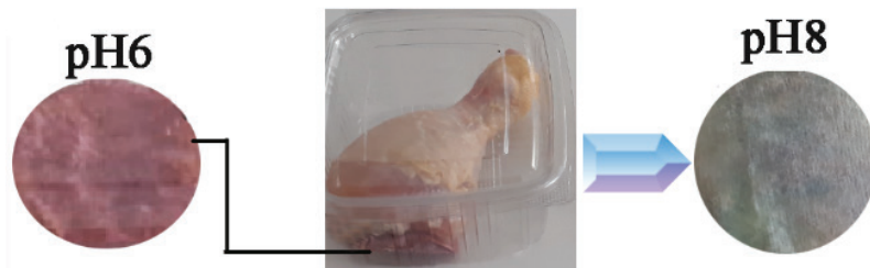
Figure 1. An indicator sensitive to pH change.
