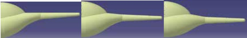
*Figure 18* Modifications on tail boom height
