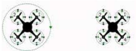
**Fig. 13.** a) All CCW propellers. b) Two CW and two CCW propellers [23]
