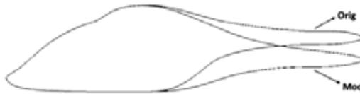
*Figure 5* Changing tail boom height, Shi et al. (2020)
