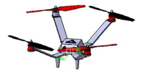
Fig. 23. Configuration 3 (Hub angle 60, arm tilt angle 30)
