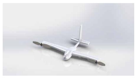
Figure 3: Rotor and wing positions of designed aircraft at cruise flight
