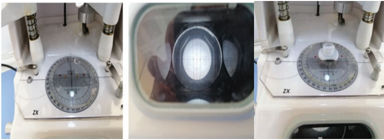
Figure 23. Optical center device, decentration adjustment and suction cups
