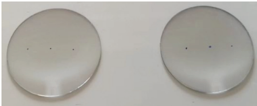
Figure 21. The marking on the lensmeter of the lenses
