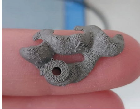
Figure 2: Printed Part with Rough Surface
