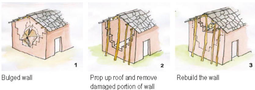
Figure 10. Steps of rebuilding a wall with out-of-plane failure (Government of Nepal National Reconstruction Authority, 2021)
