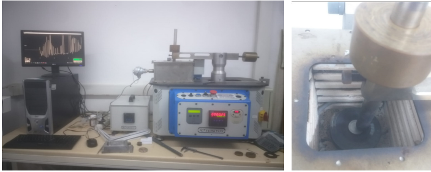
Figure 1. Wear device with high temperature chamber
