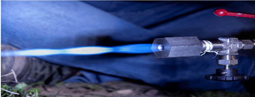
Figure 19. A thrust test of cold gas thruster in Hazar Labs.
