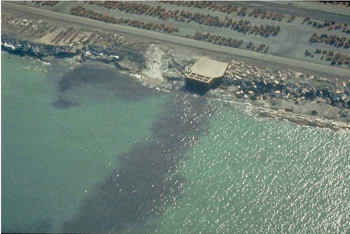
Figure 2. This image shows a point source of industrial pollution along the Calumet River. Photo: U.S. Environmental Protection Agency ( https://oceanservice.noaa.gov/education/tutorial_pollution/03pointsource.html ),
