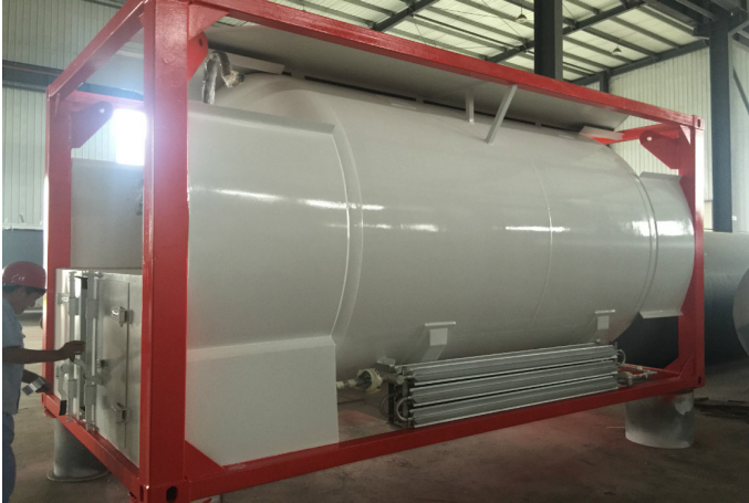
Figure 7. Liquid H_2 storage tank of Zhuhai GuangTong Low Carbon Technology.
