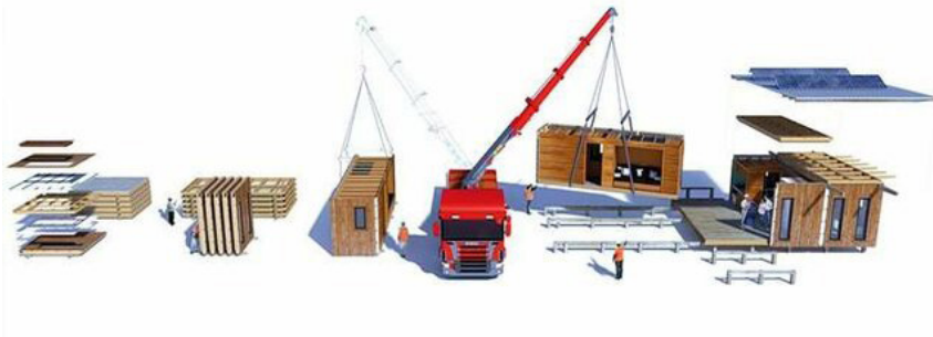
Figure 8. Production Process of Prefabricated Buildings (Patwari, 2020)
