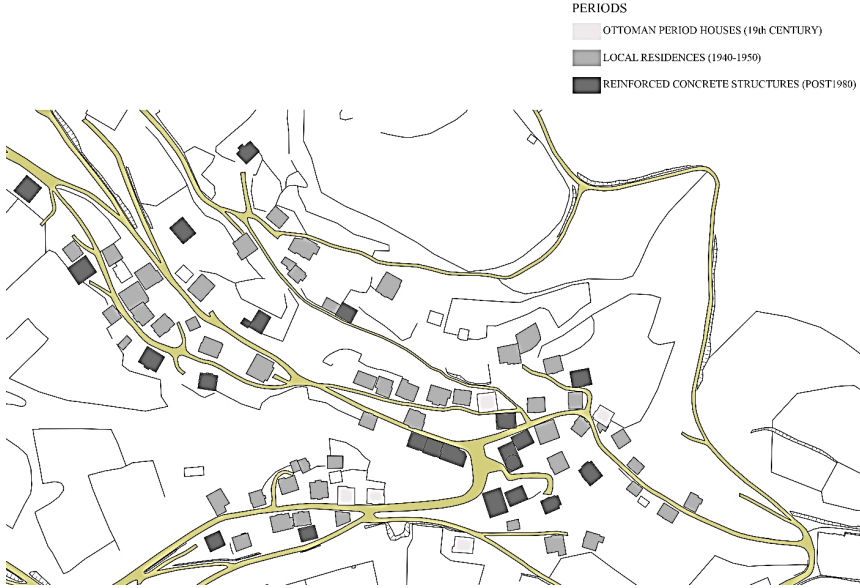
Figure 4. Distribution of houses according to construction periods
