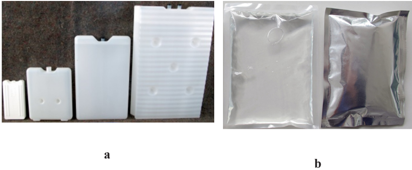
Figure 3. a) Macroencapsulation - Thermal Packages containing PCM material, b) PCM macroencapsulation: filled polymer bags
