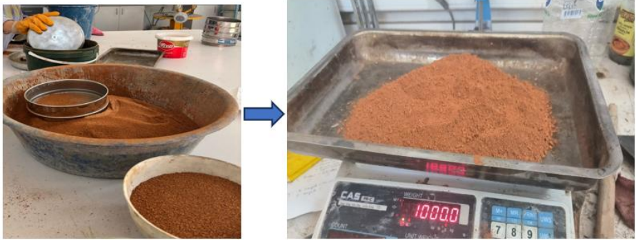
Figure 2. Preparation of brick aggregates according to appropriate granulometry
