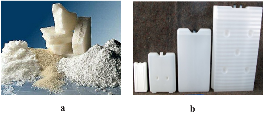
Figure 1. PCM forms available on the market, a) Powder form of PCMs, b) encapsulated PCMs (taken from https://www.rubitherm.eu/en/ )
