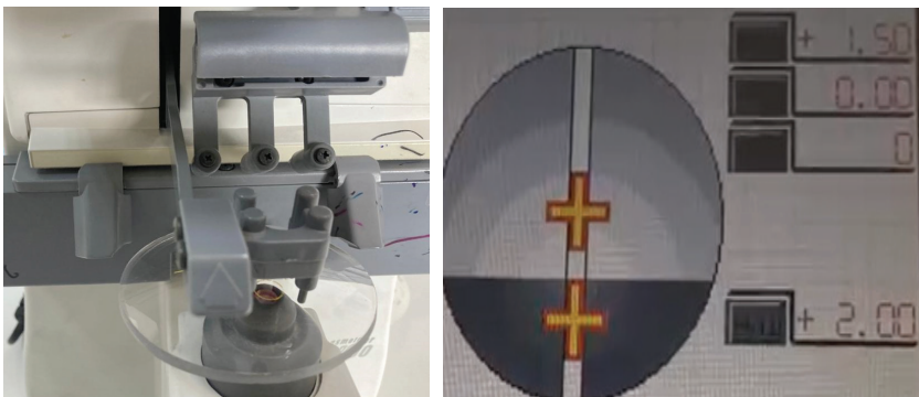
Figure 11. Diopter measurement of progressive addition lenses
