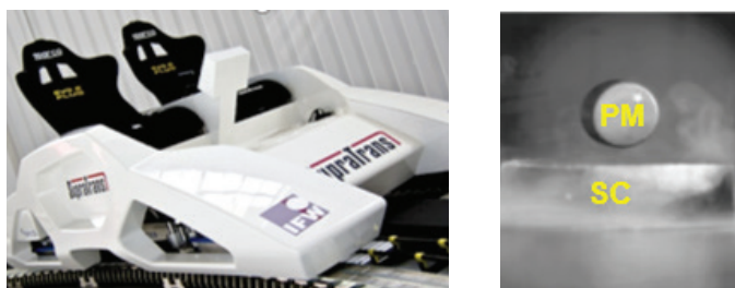
Figure 3. (a) Permanent magnet (PM) stably levitated over a bulk HTS [14], (b) The levitation of a sumo, (c) SupraTrans project, a prototype train, is an innovation transportation concept based on superconducting levitation, Dresden University, Germany [13].
