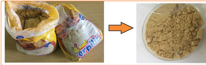
Figure 6. Micro-sized turkey feather powders (TFPs).
